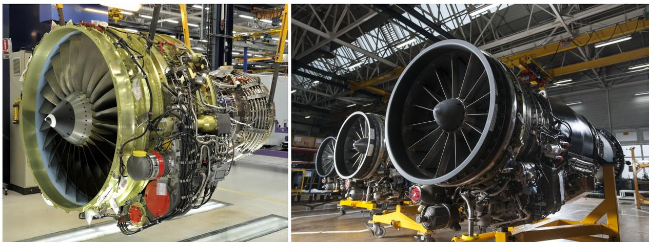
FIGURE 1.2 – Gauche: CFM56-7B. Droite: M88.
